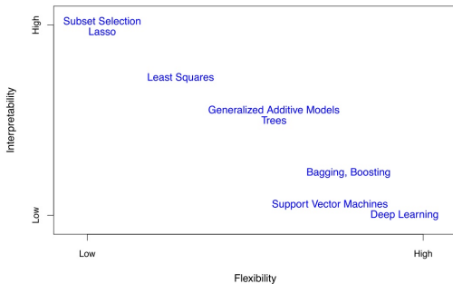
FIGURE 2.7. A representation of the tradeoff between flexibility and interpretability, using different statistical learning methods. In general, as the flexibility of a method increases, its interpretability decreases.
